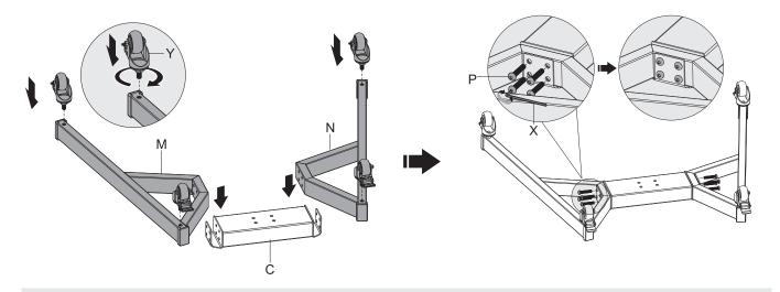
Attach the right base to the middle base and secure with screws(P). Repeat this step for the left base.
