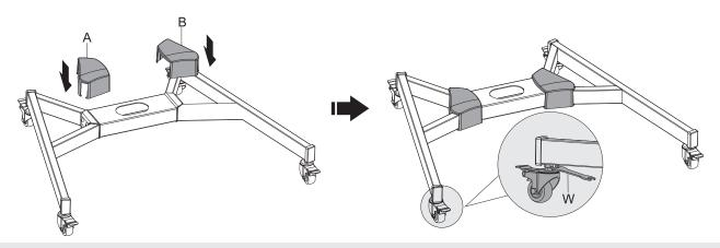
**NOTE:** Lock the brakes on the casters to avoid any sudden movements during installation.
