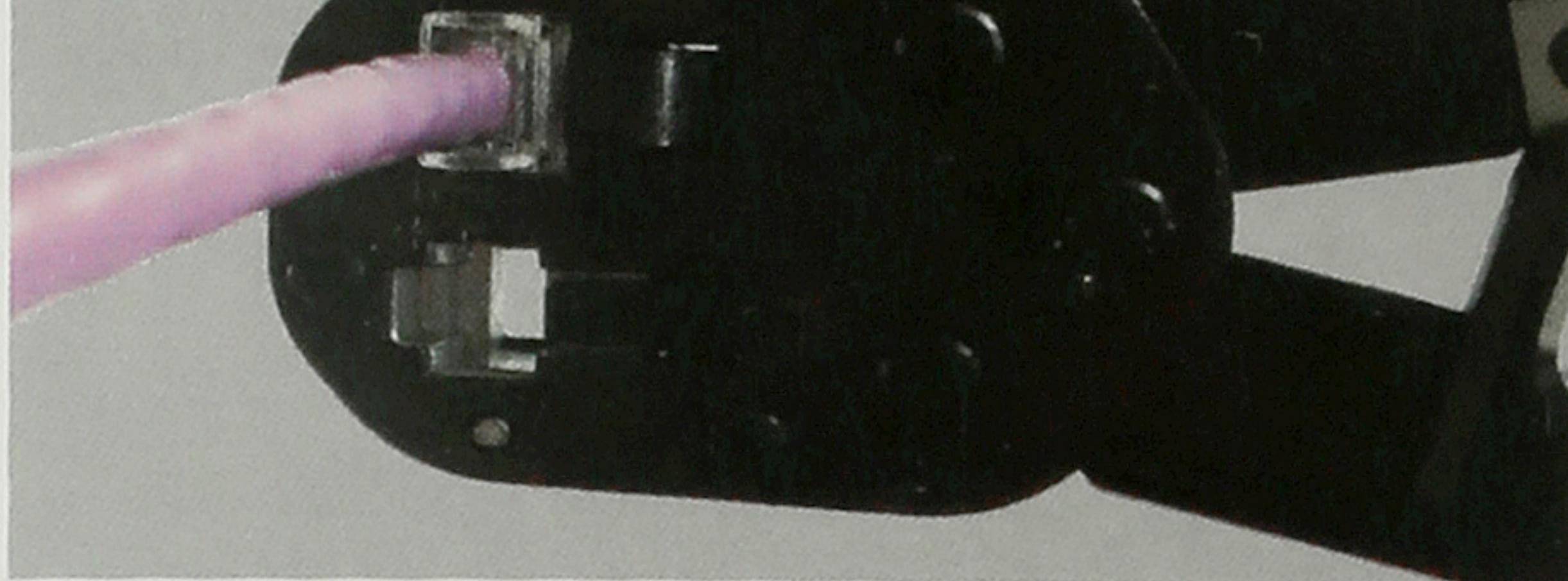
**2. Insert the plug into the correct position of the crimping tool.**
