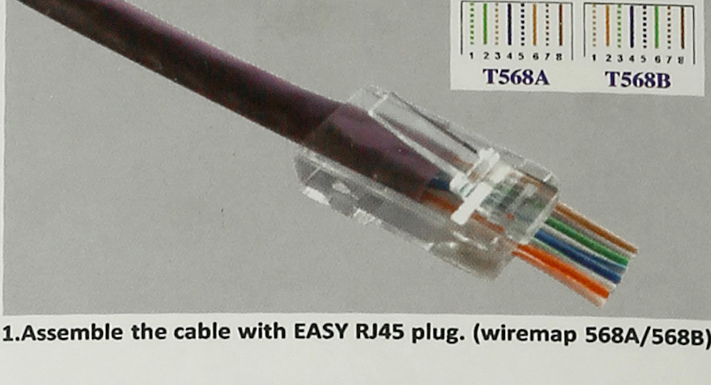
**1. Assemble the cable with EASY RJ45 plug. (wiremap 568A/568B)**
