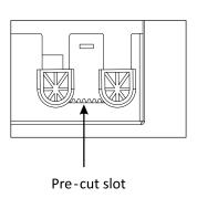
5. Run cables into box, and tight cables on cable brackets, to reduce pulling force from cable entrance edge.
